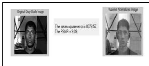
Figure 6(a) Original and Wavelet Normalized images with MSE and PSNR
